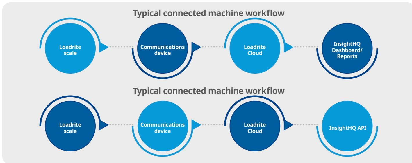
Typically, payload and production data is sent from the Communications device to InsightHQ, the messages are processed to be viewed in InsightHQ. With an API, the same time the messages can be sent through Loadrite’s API cloud and can be transferred to the customer’s connected system or database. This can happen either manually or through a batch process.
