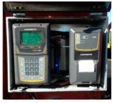
C1850 and printer protected within an enclosure
